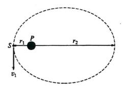
32. A satellite S is in an elliptical orbit around a planet P, as shown above, with  $r_1$  and  $r_2$  being its closest and farthest distances, respectively, from the center of the planet. If the satellite has a speed  $v_1$  at its closest distance, what is its speed at its farthest distance?
